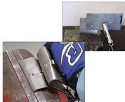
Topic D. Test Weld Destructive Testing Destructive Testing
